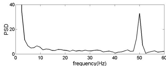
Fig. 2 Power spectrum of knee measurement. The large component under 5Hz is caused by movement and EMG.
